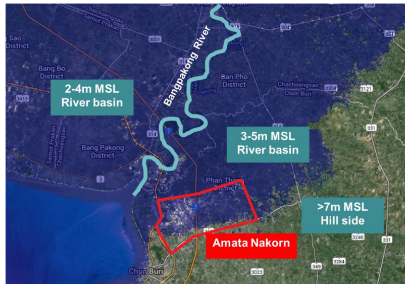
Amata Nakorn IE located in 3-5m MSL river basin The area is relatively flat
